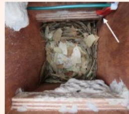
Fig. 1. Thermochron DCP210 installed in a nest box. Photo: WP3Q
